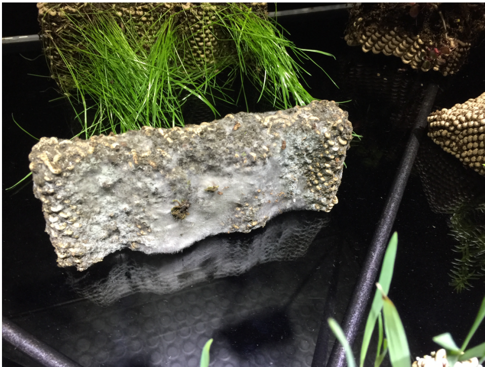
Mycelium growing through printed and fired, but not glazed clay. Collaboration with Studio UNSEEN, Tallinn Biennale. Photograph by Rachel Armstrong, 2017.
