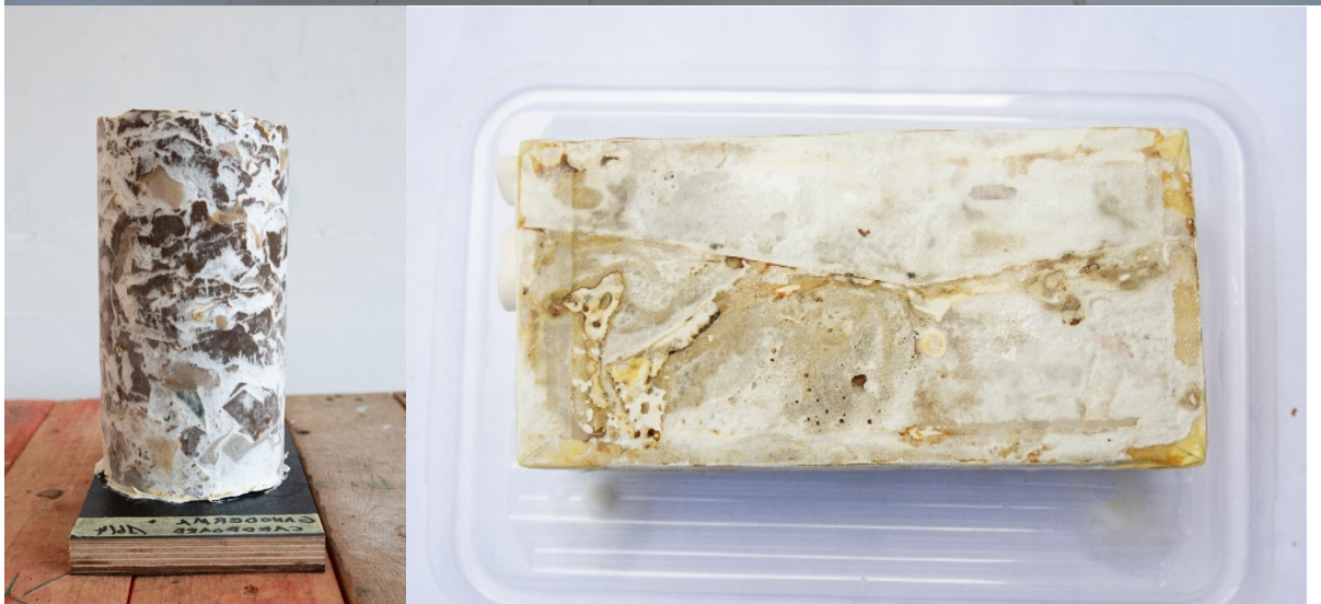
Different methods of moulding mycelium DSC07506 biocomposite using cardboard and Tupperware mould (above); PVC pipe (left) and Tupperware container (right) Samuel Hoornaerts, Wicked Home, Masters Studio, Ghent, 2022.
